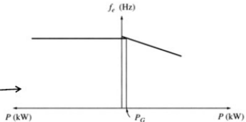
If the no-load frequency of the oncoming generator is slightly lower than the system's frequency, the generator will supply a negative power to the system: the generator actually consumes energy acting as a motor!
