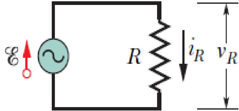
A resistor is connected across an alternating-current generator
