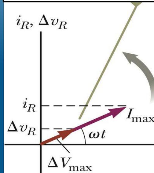
The current and the voltage in the diagram above are plotted as current and voltage phasors.
