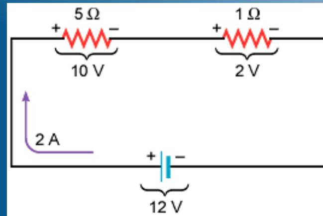
**Loop rule.** Around any closed circuit loop, the sum of the potential drops equals the sum of the potential rises.
